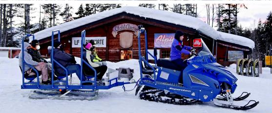
The Transalp is a solid trailer on skis, with a modular platform which can be setup in different configurations. The steel frame is coated with epoxy paint over a rustproofing base, the cargo platform is lined with a durable anti-skid diamond-plate alu layer. The frame comes already with fixing points for different set-up, light reflectors on each side, plus a 2" receiver tube on the tail for various purposes.
